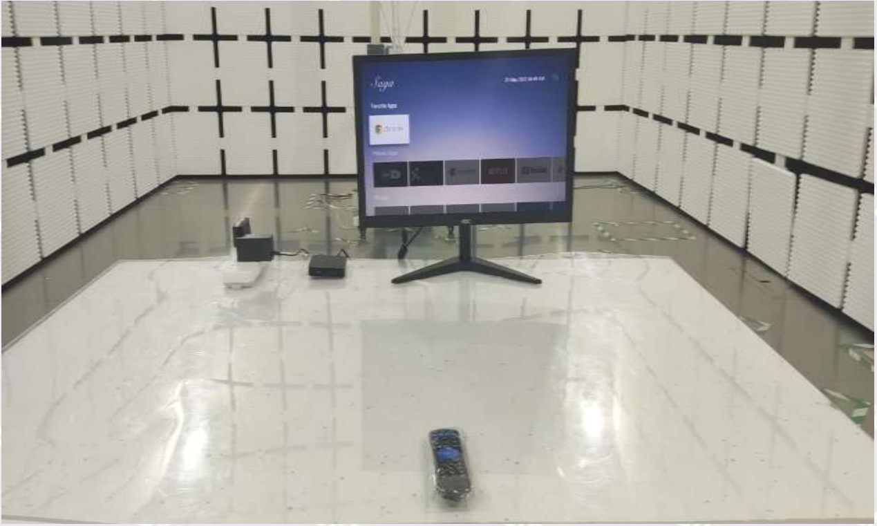
Figure 9-1 RE test setup
